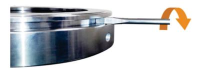
**5-**Position the shaft of the small screwdriver as a wedge over DOT 1, lean the large screwdriver over the shaft of the small screwdriver and repeat step 4.
