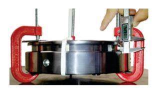
**6-**Gently turn the 3 adjustment shafts of the "C" clamps (one at a time).
