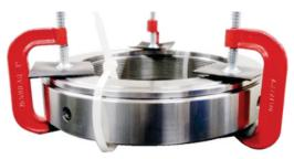
**7-**Remove the nylon clamps and check if the Piston fully abuts the nut.
