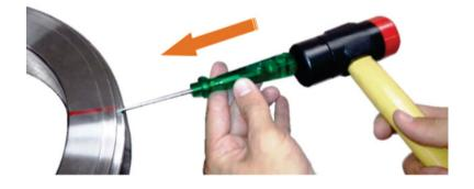
**3-**Introduce again the small screwdriver into DOT 1 and turn the driver so to displace the Piston, as shown by the next figure. Repeat the operation for DOTS 2 and 3.
