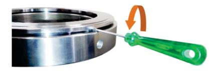
**4-** Position the large screwdriver ono DOTS 1, 2 and 3 and, turning the driver, displace the Piston in appropriate balance until fully displacing it.
