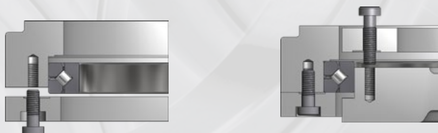
Mounting Crossed roller bearing with clamping rings
