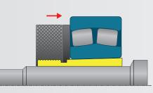
b Connect the pump to the HMV.
